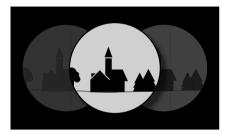
Adjust the interocular distance by moving the hinged joint to match your personal requirements. When the interocular distance is set correctly, the right and left fields of view merge into a circular image.
