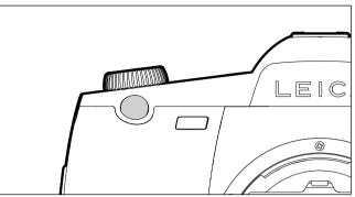
The shutter button works in two stages.
