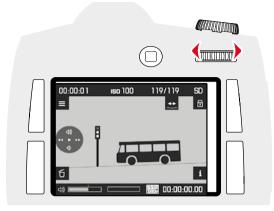
Use the thumbwheel to access other saved pictures. Once the first/last picture is viewed, the image series starts again in an endless loop accessible in both directions. The picture numbers change accordingly.
