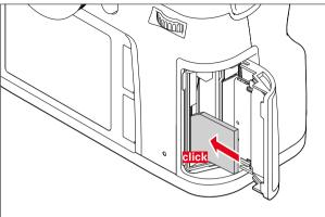
Memory card - with the contacts facing towards the rear and the beveled corner facing upwards - push the card in fully against the resistance of the spring until it clicks into place
