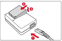
A properly operating charging process is indicated by the status LED lighting up. The battery will be fully charged when the green LED switches off.
