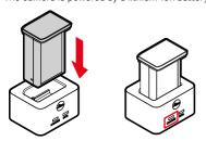
The status LED indicates a correct charging process.
