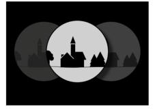
Adjust the interpupillary distance by moving the hinged joint to match your personal requirements. When the interpupillary distance is set correctly, the right and left fields of view merge into a circular image.
