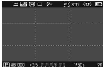
3.2" TFT LCD, 1080 x 720 pixel, circa 2 332 800 pixel (dot), display touchscreen
