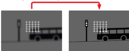
After the setting has been made, the metering fields are displayed in which the subject sections are displayed in focus.
