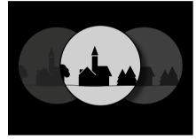
Adjust the interocular distance by moving the hinged joint to match your personal requirements. When the interocular distance is set correctly, the right and left fields of view merge into a circular image.
