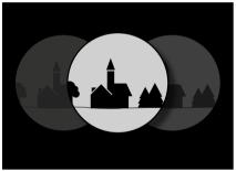
Adjust the interocular distance by moving the hinged joint to match your personal requirements. When the interocular distance is set correctly, the right and left fields of view merge into a circular image.
