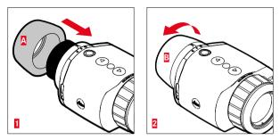
The eyecup supplied must be attached if the device is to be used as a handheld/monocular (without the rifle scope).
