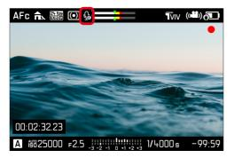
The use of an external USB microphone requires an activation of the function via the menu. Once the function USB Microphone is activated, the camera will automatically switch from the internal to the external microphone.
